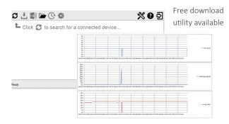
The VAPex can store up to 200 separate runs, storing data including start time, stop time, date, duration, volume sampled and motion index.
